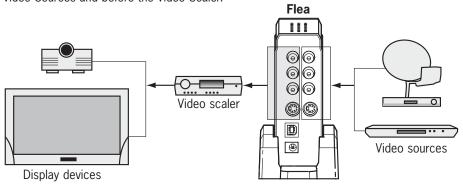
• To enhance your Home Theatre listening experience, the **Flea** is fanless and achieves cooling through natural convection and dissipation of heat. Therefore, when installing the **Flea**, do not obstuct any of its air vents, nor place it over heat dissipating devices such as amplifiers. Placing the **Flea** near heat sources can damage it or cause it to overheat and not operate properly.
